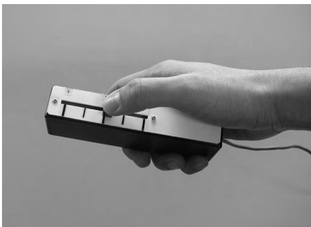
Fig. 3. Continuous rating device to output participants' feelings of pressure.
